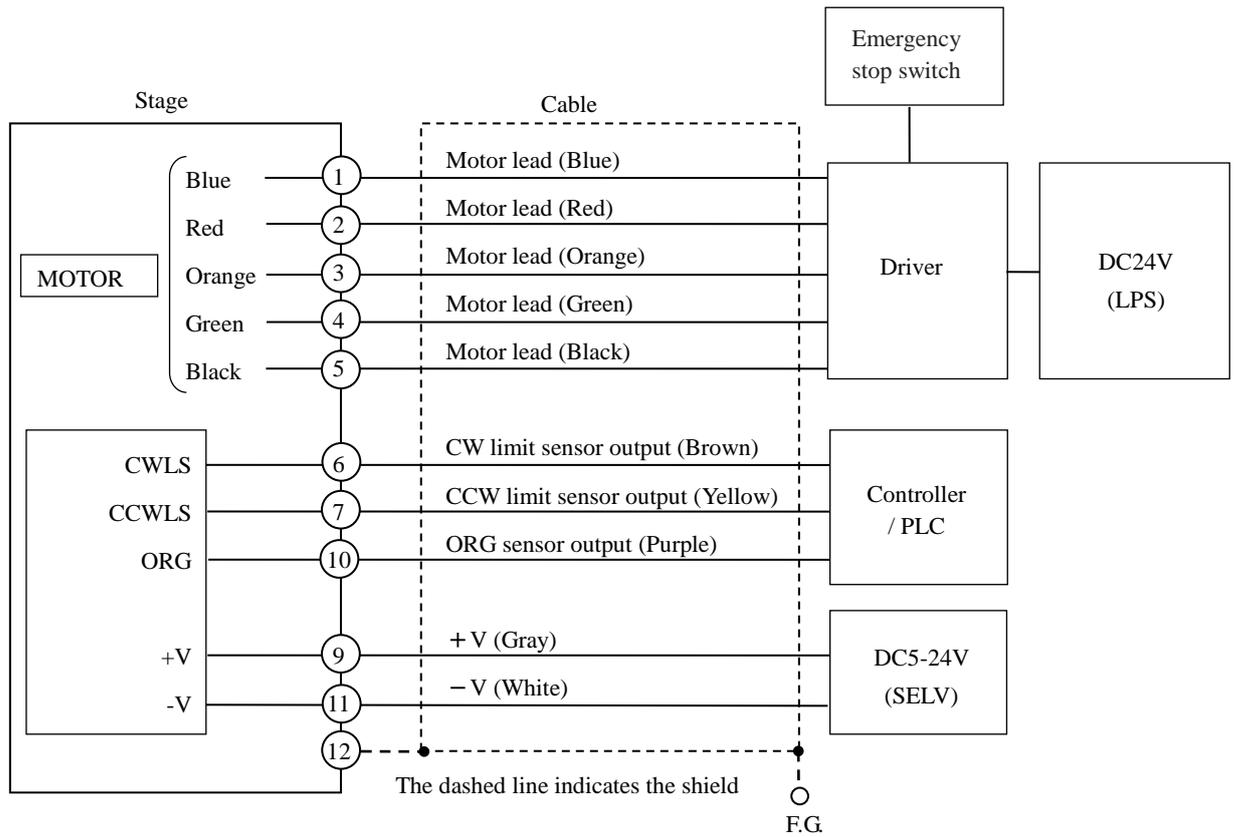
\* Install an emergency stop switch on the power supply of the driver.
