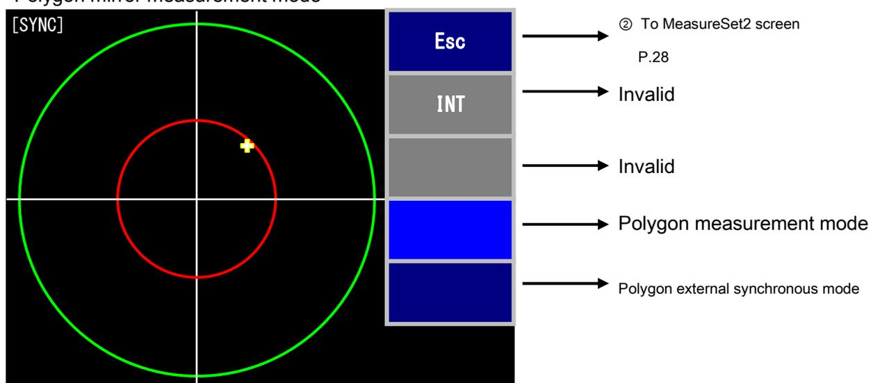
\* When the polygon measurement mode is selected, EXT2 (face detection signal) is automatically selected.
