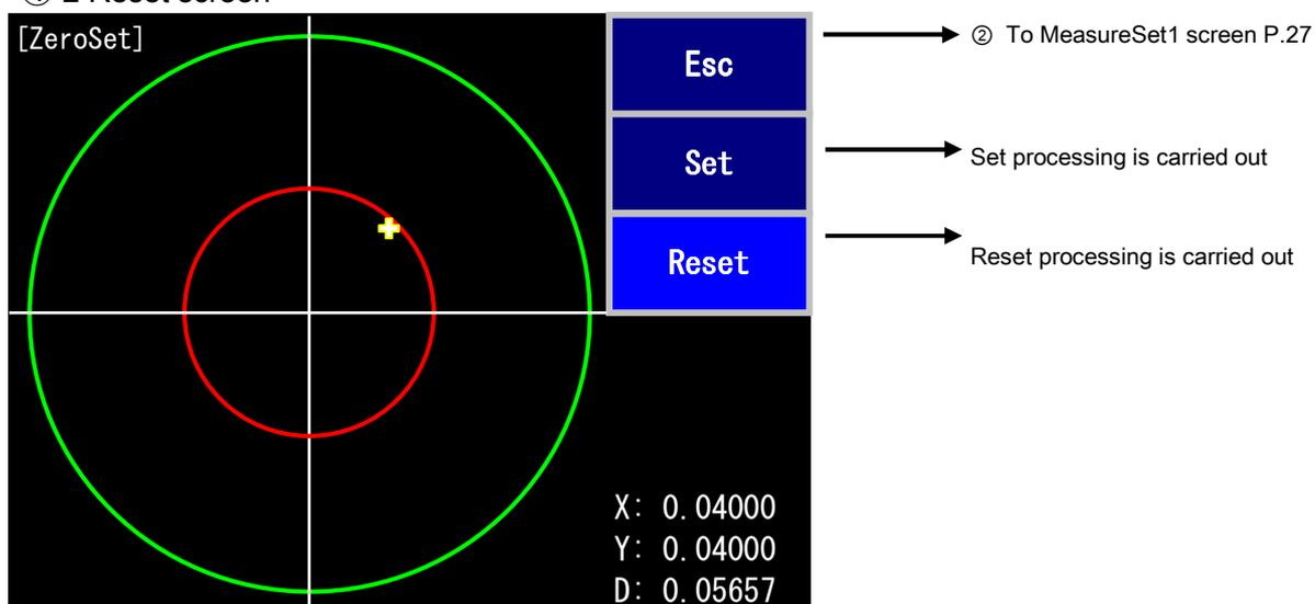
Reset button: The measurement standard is set to the measurement origin (center of screen).
