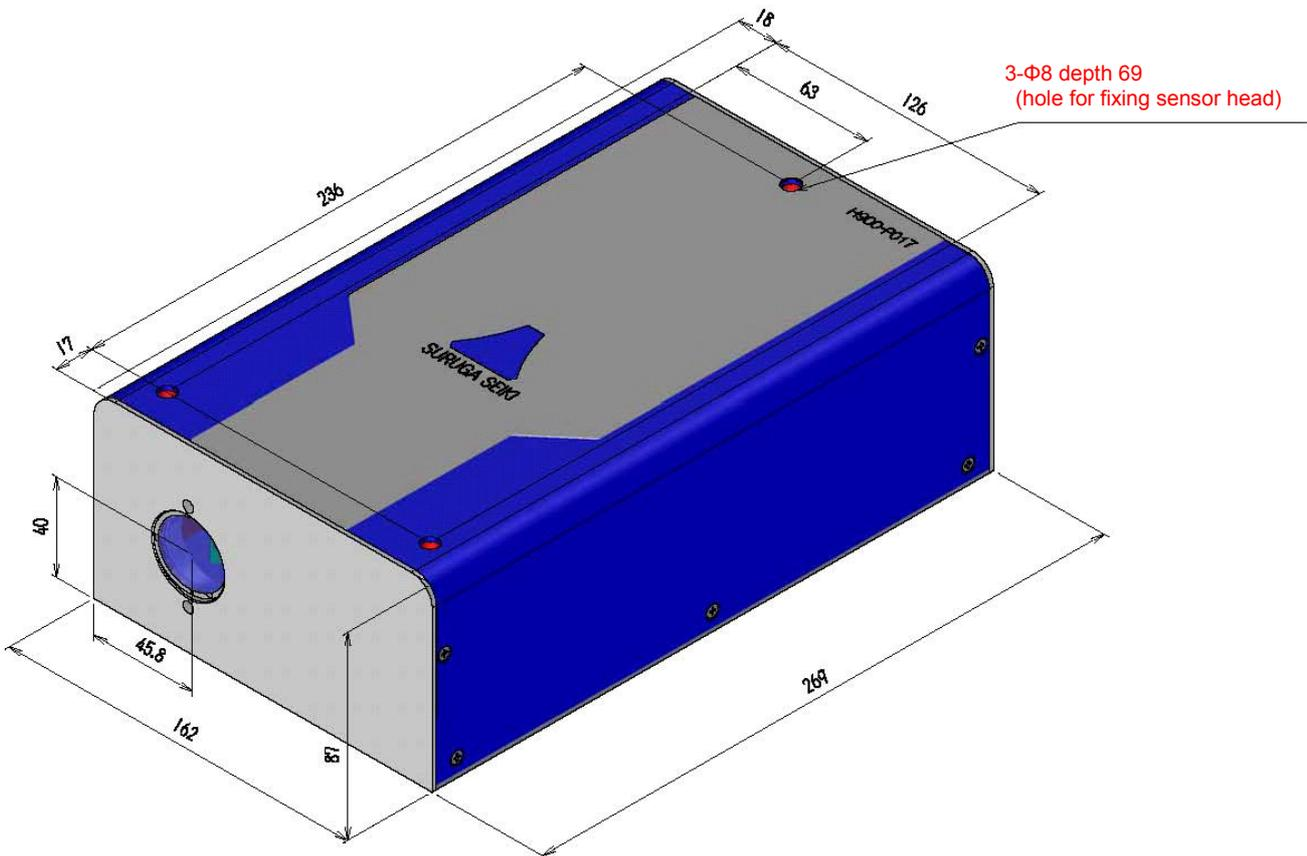
\* For the bolt used for the sensor head fixation hole, use the bolt whose length is longer than that of hexagon socket bolt M4x25 (3 pieces).
