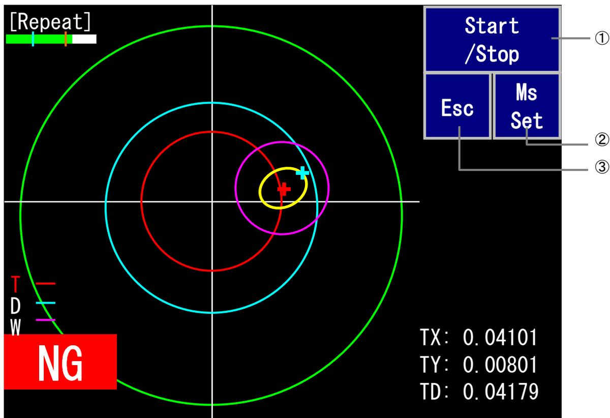
\* If the measurement is stopped during measurement by Stop button, Stop I/O or Stop command, the measurement is stopped after 4096 sample data are obtained.
