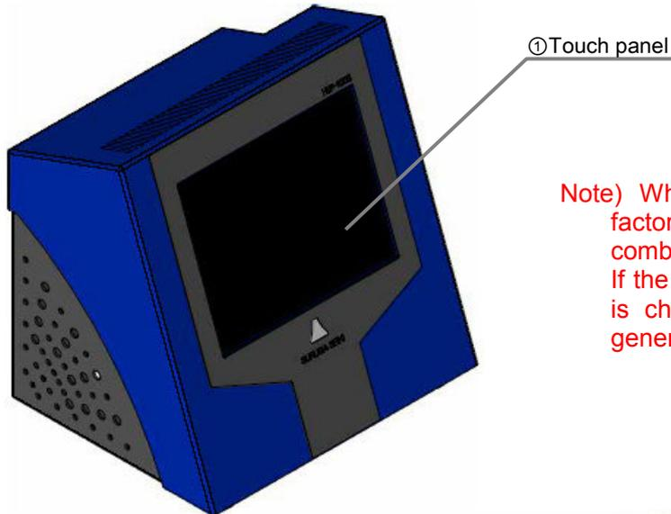
Note) When the product is shipped from factory, the calibration is carried out in combination of head and controller. If the combination of head and controller is changed, the measurement error is generated.
