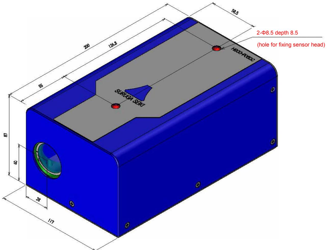
\* For the bolt used for sensor head fixation hole, use the bolt whose length is longer than that of hexagon socket bolt M4x25 (2 pieces).
