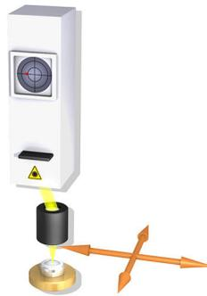
Optical axis adjustment is available in LD mounting process. By direct insertion of the light from LD, measuring inserted light can be achieved. Power off the light from Auto collimator and Auto collimator needs to be placed as base line. During measuring internal light source needs to be off
