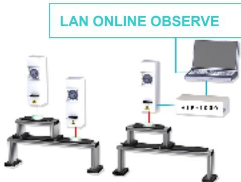
Available to measure the inclination and parallelism of surface table, parts etc.
